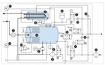
1 2-2 way valve (normally closed), 2 circulation pump with reversible pumping direction, 3 tube bundle heat exchanger, 4 heating element, 5 filter, 6 expansion vessel, 7 flow sensor, 8 level sensor, 9 temperature sensor, 10 thermostat, 11 pressure gauge, 12 pressure relief valves, 13 non-return valve
