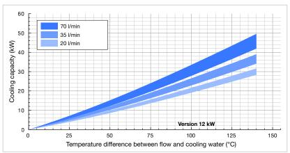
Power specifications 12 kW at min. 12 l/min @ 2 bar; at max. 25 l/min @ 8 bar cooling water
